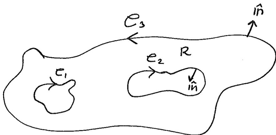
Green's theorem still holds with proper orientation of the boundary  $\partial R = C_1 + C_2 + C_3$
